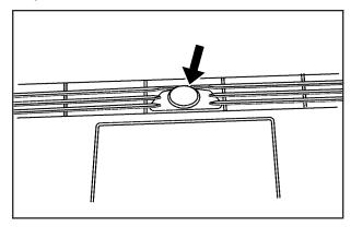
A light sensor on top of the instrument panel makes the Twilight Sentinel® work, so be sure it is not covered.
